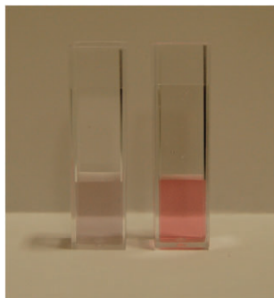
Fig. 4 Photograph of nanoparticle probes obtained 1 hour after addition of double stranded DNA. Left cuvette: complementary target; right cuvette: target incorporating a single base pair mismatch.
